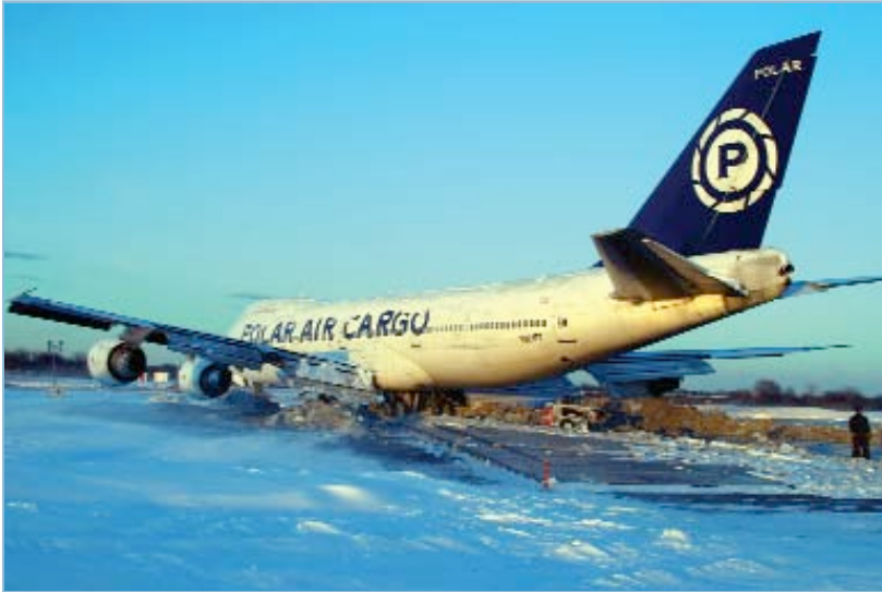
EMAS system stops Boeing 747 that overran the runway at JFK Airport on January 22, 2005.
